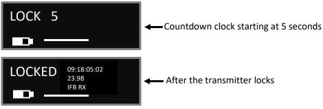
This page enables a key lock function so no parameters can be changes. When the lock page is landed on a countdown clock will begin. After 5 seconds the TRXCL5 will lock, and the display will indicate that it is LOCKED. If this screen is exited before the 5 seconds are up the transmitter will not lock.
