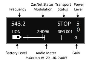
**Frequency** - This is the transmit frequency of the ZMT4.
