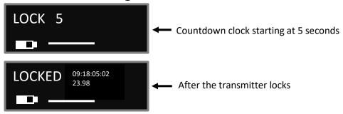
This page enables a key lock function so no parameters can be changes. When the lock page is landed on a countdown clock will begin. After 5 seconds the transmitter will lock, and the display will indicated that it is LOCKED. If this screen is exited before the 5 seconds are up the transmitter will not lock. When the transmitter is locked the OLED will turn off.
