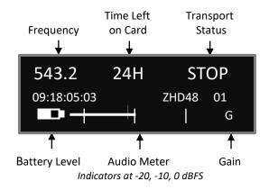
**Frequency** - This is the transmit frequency of the ZMT4 Flex.
