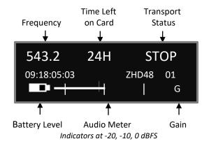
Frequency - This is the transmit frequency of the ZMT3-X.
