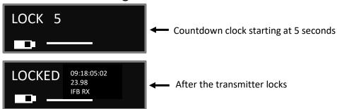
This page enables a key lock function so no parameters can be changes. When the lock page is landed on a countdown clock will begin. After 5 seconds the transmitter will lock and the display will indicated that it is LOCKED. If this screen is exited before the 5 seconds are up the transmitter will not lock.
