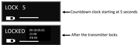
This page enables a key lock function so no parameters can be changes. When the lock page is landed on a countdown clock will begin. After 5 seconds the TRXCL4 will lock, and the display will indicate that it is LOCKED. If this screen is exited before the 5 seconds are up the transmitter will not lock.
