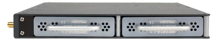
The two MRX receivers slide into the side of the RX-8. The A receiver goes to in the bottom slot away from the front panel and the B receiver goes in the top by the front panel. The arrows on the MRX will need to point to the bottom of the RX-8. Please note if only using 1 receiver it must go in the A slot.
