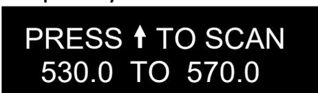
The frequency scan menu is where the A receiver of the RX-4 can scan the user specified frequency range and search for a clear frequency. After the scan is complete a graphical display of the RF that is present, in that specified range will be shown and the RX-4 will suggest a clear frequency. That frequency can be accepted by pressing the INC key. Or press the DEC key to skip the first chosen frequency and have the RX-4 suggest another frequency.
