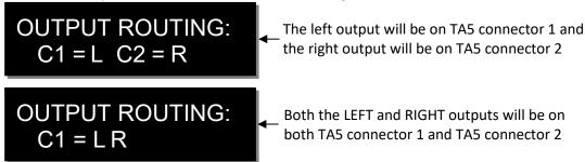
This menu sets the output assignments of the TA5 connectors when the QRX is set to single mode and is receiving a signal from a stereo transmitter.
