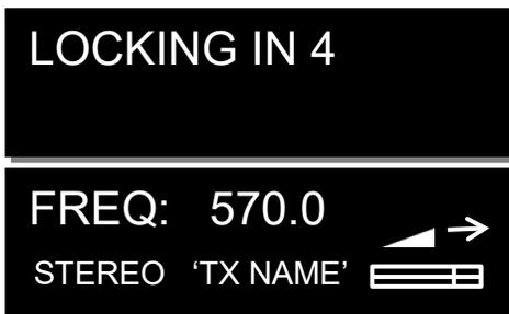
The lock screen is landed on a 5 second countdown clock will start. After 5 seconds elapse the URX100 will lock and the menus cannot be accessed. This is to prevent the parameters from accidentally be changed.
