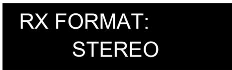
The modulation menu is where the receive format is set. Modulation is simply the way a transmitter “modulates”, or sends, its signal to the URX100. This setting needs to match the modulation mode that the corresponding transmitter is set to - if the two settings do not match the URX100 will not be able to receive and decode the signal from the transmitter.
