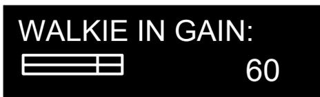
The walkie in gain menu is where the level of the optional lanyard microphone input from to the URX100 is set. The higher the level is set the more gain the microphone will have.
