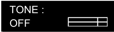
The tone menu allows the URX100 to output tone. This is useful to set levels and check routing. Pressing the CH UP and CH DOWN keys will cycle through and output the different tone settings.
