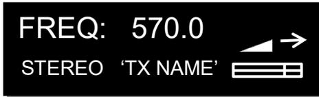
The frequency select menu is where the URX100 receive frequency is set. This frequency needs to match the frequency that is set on the corresponding transmitter. To adjust the frequency press the channel up key to increase the frequency and press the channel down key to decrease the frequency. Also displayed is the modulation format, the name of the transmitter being received, a signal strength meter and audio meter and an arrow showing which antenna the signal is being received on.
