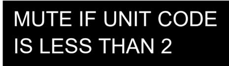
This menu sets if transmitters with certain ZaxNet unit codes will not be able to be monitored by the URX100. For example if this menu is set to 30 any transmitter with a ZaxNet unit code below 30 will not be able to be monitored by the URX100.
