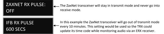
This menu sets the interval that the ZaxNet transceiver will stop sending confidence audio and search for time code.
