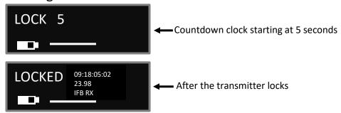
This page enables a key lock function so no parameters can be changes. When the lock page is landed on a countdown clock will begin. After 5 seconds the TRXCL3 will lock and the display will indicated that it is LOCKED. If this screen is exited before the 5 seconds are up the transmitter will not lock.
