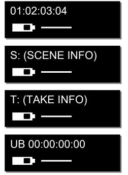
The main screen of the ERX will display timecode, battery level and receive audio level.
