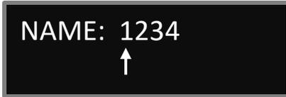
The transmitter name menu allows the transmitter to be named to be changed from the default name - which is the unit's serial number. The name entered becomes part of the name of the recorded audio files, and is also included in the metadata of the BWF file. Naming the unit aids in identifying the files from several different recorders.
