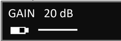
The microphone gain is adjusted from this menu. This menu displays the gain setting in decibels and a meter indicating the audio signal. The meter is displayed horizontally from left to right.
