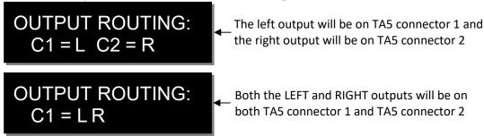
This menu sets the output assignments of the TA5 connectors when the QRX is set to single mode and is receiving a signal from a stereo transmitter.
