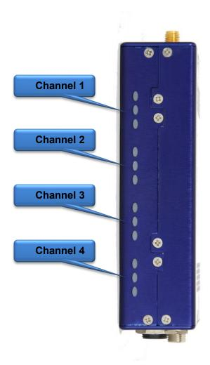
**Side Mounted LEDs** - The LEDs give visual indication if RF and / or audio are being received by the QRX. The LED settings are adjusted in the extended menu. There are three LEDs per group and one group for each receive channel. The group to the top represents channel one, the group below is channel 2, the next group is channel 3, and the group on the bottom is channel 4.
