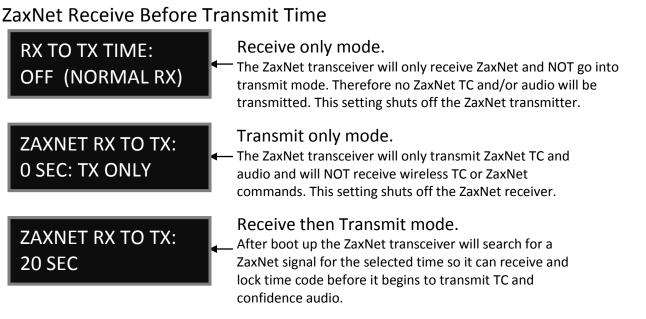
This menu adjusts the state of the ZaxNet transceiver. This also sets how long after boot-up up the TRXLA3 will search for ZaxNet time code before it begins transmitting its audio over ZaxNet for monitoring purposes. This is so the TRX3LA can lock to ZaxNet time code source before the unit will send confidence audio over ZaxNet.
