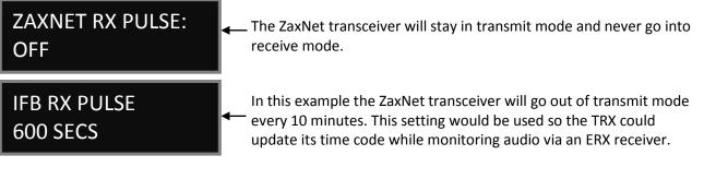
This menu sets the interval that the ZaxNet transceiver will stop sending confidence audio and search for time code.
