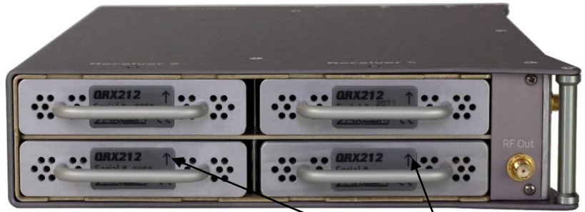
QRX212 Modules slide into the RX12 with the arrow pointing to the top of the RX12
