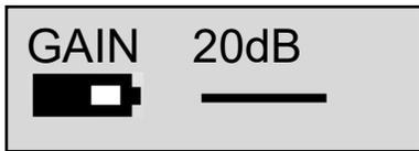
The microphone gain is adjusted from this menu. This page displays the gain setting in decibels and a meter that indicates the audio signal. The meter is displayed horizontally from left to right.
