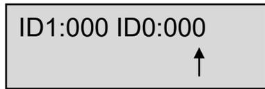
If the encryption code is turned on the ZaxNet transmitted audio will be encrypted and can only be listened to if the receiver has the matching encryption code entered. When receiving an audio signal and the codes do not match, all that will be heard is white-noise or silence. So if using encryption make sure the matching receiver has the same code.
