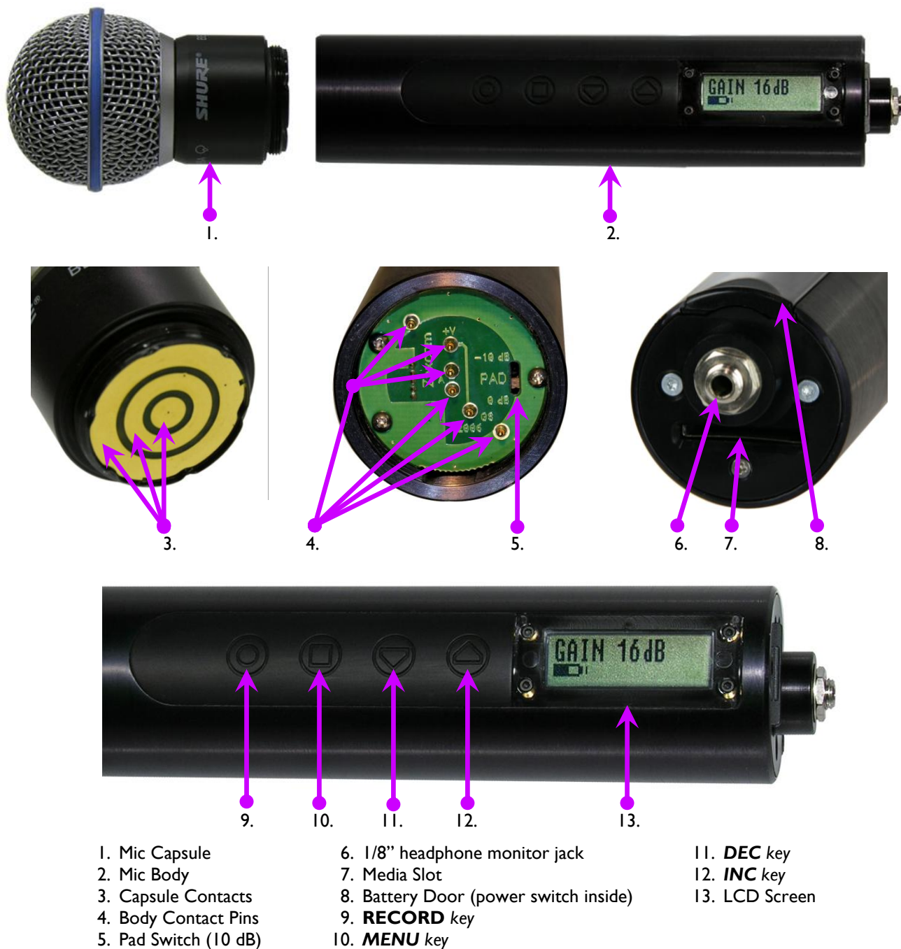
Figure 2-3 ZFR800 Side, Mic Capsule, Body Threaded End, Body Antenna End & Body Side Views
