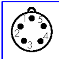
Figure 10-5 LEMO-5M Timecode Connector Pin Numbering
